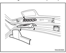
To replace a center high-mounted stop lamp bulb:
